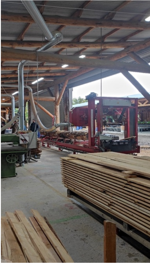
Photo 10 & 11: (L) Stenner bandsaw sawmill (R) Wadkin Table saw. Traditional timber frame joinery construction on roof and walls
